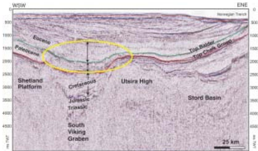
**Figure 2** Regional seismic cross-section showing the location of remobilised and injected fields (within yellow outline) in relation to the main structural and stratigraphic elements of the northern North Sea (~60°N). Location of seismic line is shown on Figure 1.
