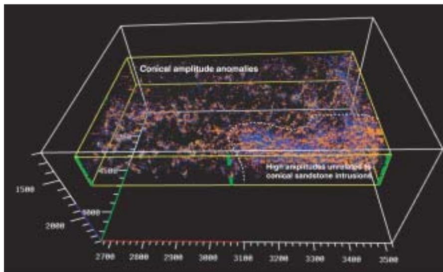
**Figure 8** Volume visualisation showing the pervasive occurrence of conical amplitude anomalies in the Lower-Middle Eocene of the South Viking Graben. All but the highest positive and negative amplitudes are rendered transparent. The volume is about 18 km wide, 12 km deep and 400 ms TWT high.
