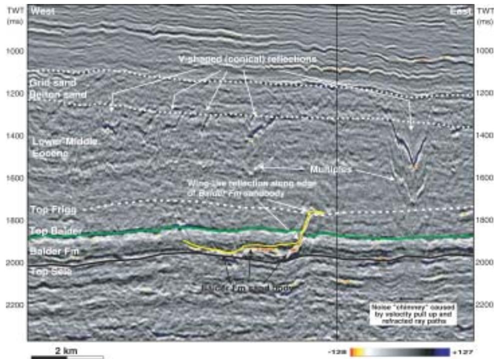
**Figure 5** Conventional P-wave seismic section showing the two major classes of seismic-scale injection features: Wing-like amplitude anomalies (low-angle sandstone dykes) emanating from the sides of steep-sided sandbodies and conical amplitude anomalies (conical sandstone intrusions) detached from underlying sandbodies. Figure modified from Huuse et al. (in press). Location of seismic line is indicated on Fig. 7
