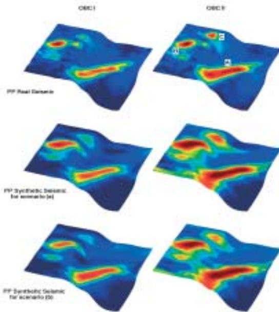
**Figure 7** Comparison between PP real and synthetic amplitude maps for OBC I and OBC II. The amplitudes are in agreement with what is observed in the real data. Anomalies B and C show time-lapse signature due to production from the main reservoir as pressure depletes through a pressure communication path. The anomalies B and C for scenario S1 are 20% brighter than those of scenario S2, which is what is observed in the real data.
