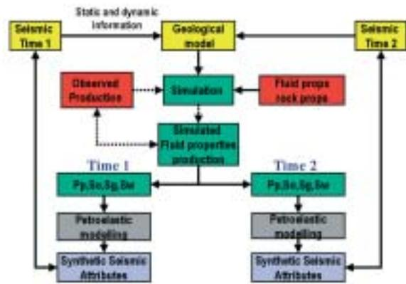
**Figure 4** Flowchart showing the procedure for 4D-4C seismic history match which includes production history match. The simulated saturation and pore pressure are used to generate time-lapse synthetics using 1D AVO seismic modeling for both PP and PS via petroelastic modelling.
