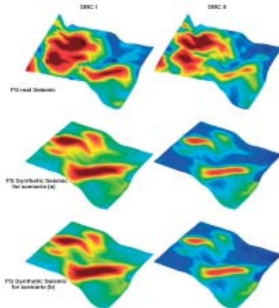
**Figure 8** Comparison between PS real and synthetic amplitude maps. There is a decrease in amplitude between the two surveys consistent with what is observed in the real data. The undrilled area (anomalies B and C) has a difference in character between real and synthetic seismic.
