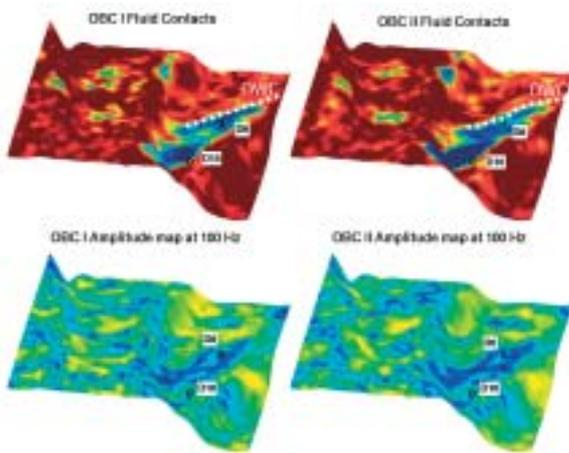
**Figure 3** Fluid contact and amplitude maps at 100 Hz, after spectral decomposition, for OBC I and OBC II. Between the two surveys, the expansion of gas cap and movement of OWC could be observed. The channels within the turbidite sand can be clearly seen on the amplitude map. These could be high NTG channels incised in the turbidite sheet.
