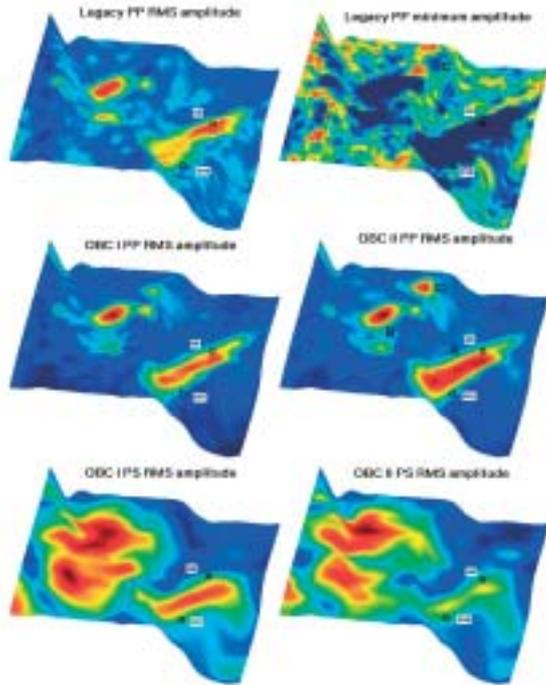
**Figure 1** PP amplitude maps for towed-streamer and PP and PS maps for OBC surveys. Time-lapse anomalies A, B and C are identified on OBC I and II. Anomaly C that cannot be seen on RMS amplitude map can now be seen on minimum amplitude map of the towed-streamer legacy data.
