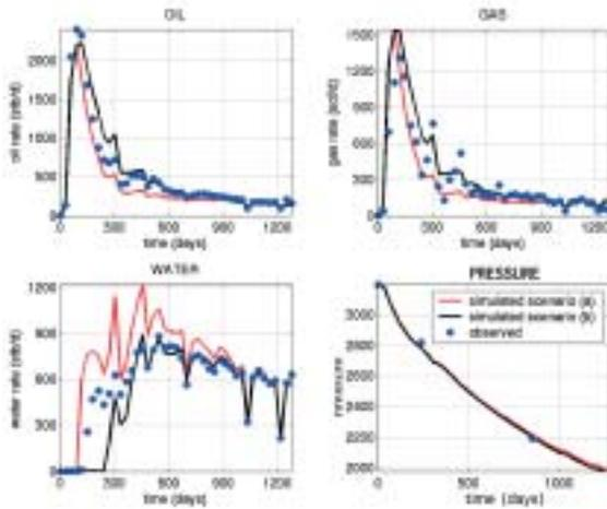
**Figure 6** Production history match for Teal South for both scenarios. The red line denotes the simulated production for scenario S1, black line denotes the simulated production for scenario S2 and the blue dots represent the actual production. For both scenarios, there is good match between the simulated and the actual production.
