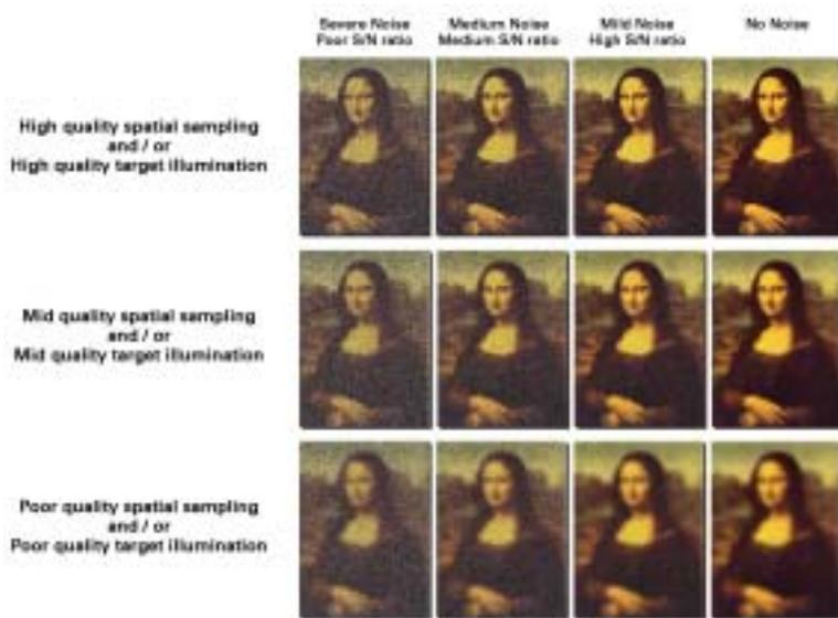
Figure 1 A demonstration of the irrelevance of S/N ratio, when pursuing the ultimate imaging quality. When S/N ratio is poor, an inherently high quality signal is quite indistinguishable from a low quality signal. However, as S/N ratio improves, we begin to recognize that other underlying factors than the uncorrelated noise envelope affect the degree to which signal resolution and quality can be achieved.
