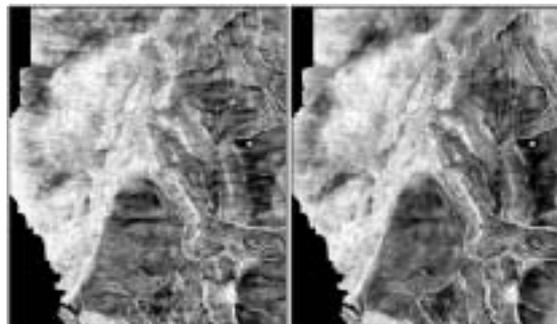
**Figure 4** Comparison of base Cretaceous (target) amplitude maps for 3D seismic data acquired in one direction (left: 270/90° acquisition) vs. 3D seismic data composed of three directions (right: 270/90°, 150/330°, and 30/210°). Both the acquisition footprint and other processing artifacts are greatly decreased on the right (multi-azimuth HD3D acquisition), demonstrating how pre-stack imaging benefits from improved azimuthal sampling and illumination.
