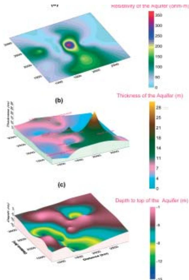
Figure 4 3D maps prepared after interpretation of the VES data: (a) true resistivity contour map; (b) thickness; (c) depth to the top of the aquifer.
