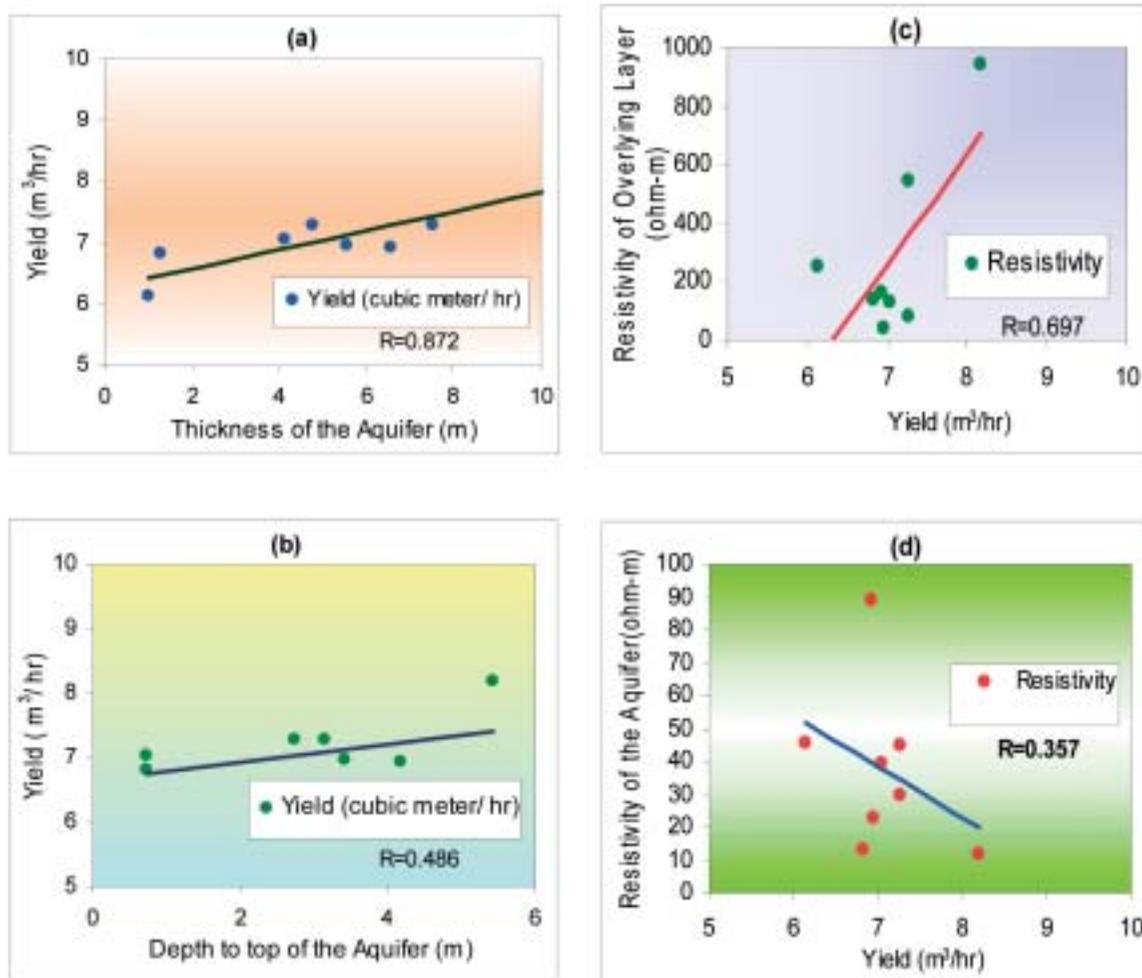
Figure 5 Correlation study of the yield of the aquifers with (a) thickness, (b) depth to the top, (c) resistivity of the overlying layer and (d) resistivity of the aquifer.
