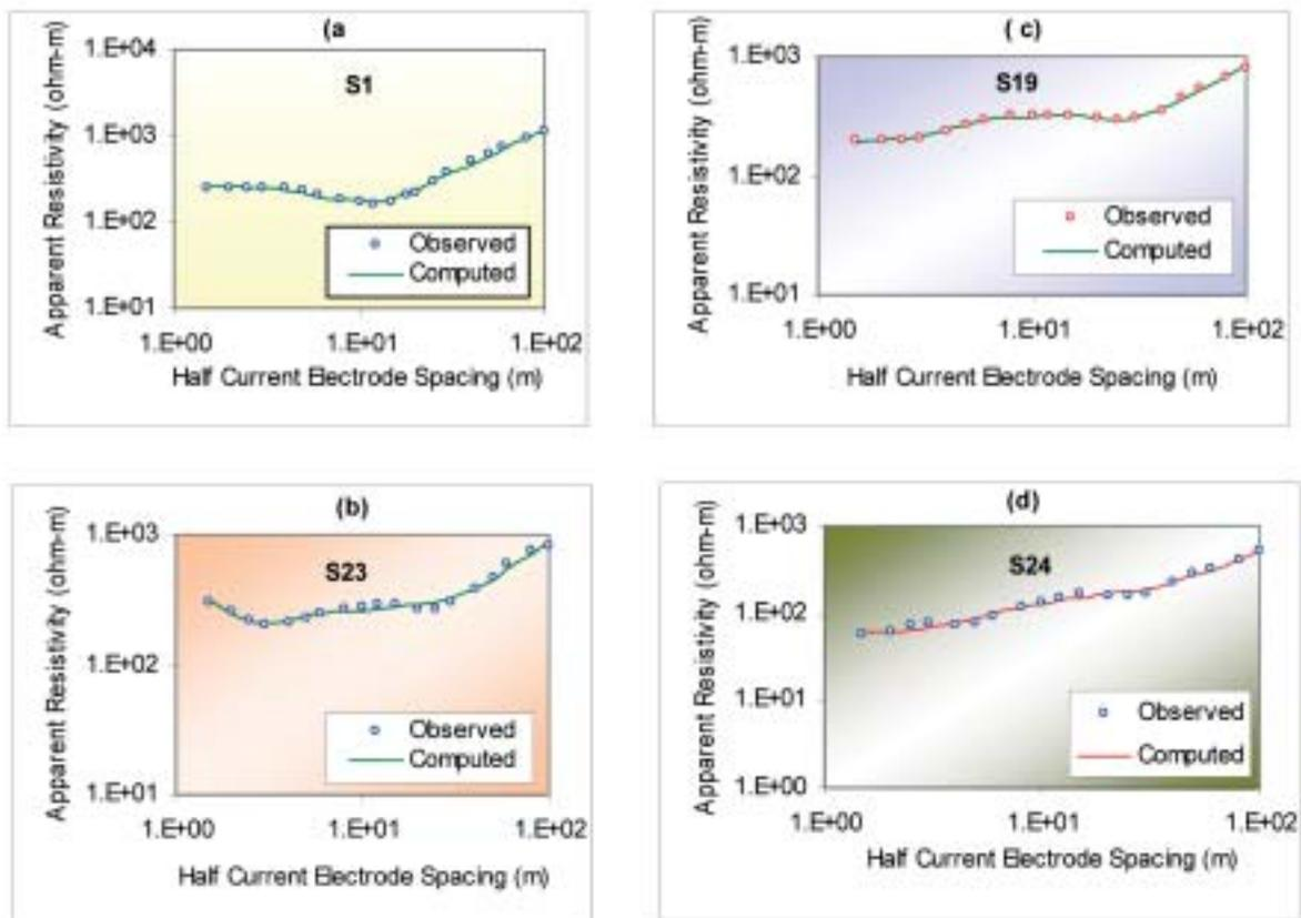
Figure 3 Some typical observed and computed VES curves obtained after inversion of field data.
