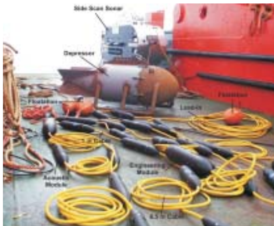
Figure 2 Photograph of the deep-tow system components, prepared for deployment from the ship's stern during RV Sonne cruise SO162. Front: streamer nodes and cables, middle: 2 tons depressor, back: sidescan sonar towfish.
