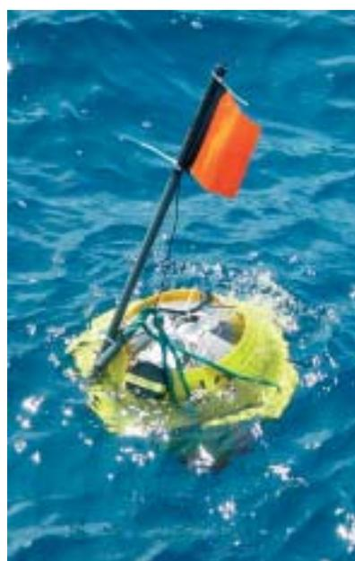
Figure 12 An OBS. All the OBS used were four component (three component seismometer and a hydrophone).
