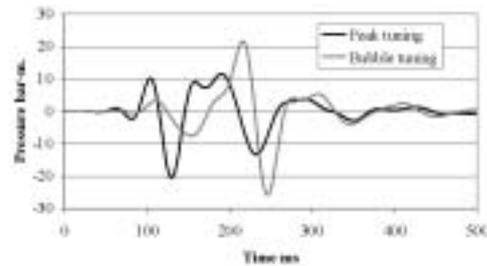
**Figure 6** Pre-survey modelled signatures for peak and bubble tuning after the application of a 20 Hz, zero-phase, low pass filter. The bubble-tuned signature is more compact and has a greater peak-to-peak amplitude.
