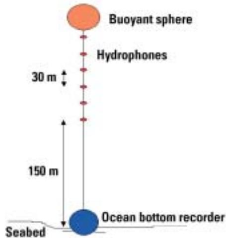
Figure 8 A schematic diagram of the vertical hydrophone arrays. Each consisted of a heavy ocean bottom recorder, 300m cable, 6 hydrophones and a buoyant sphere deployed as shown.
