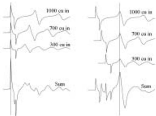
**Figure 5** Left: tuning on the peak. Right: tuning on the bubble.
