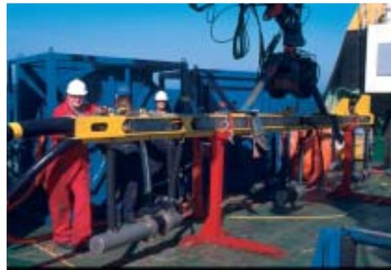
**Figure 7** Two of the beams used (one is barely visible). The closest gun is 700 cubic inches in volume; the beams were deployed over the side using the crane at the top of the picture.
