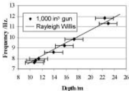
Figure 2 Observed bubble frequency-depth data.
