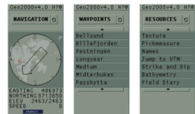
Figure 3 The interface is very simple and intuitive in use. Left menu is a navigator, informing the user of position, view elevation and speed when 'flying'. Middle menu lists waypoints, or placed where local data (resources) are available. When clicking on a waypoint, the simulator automatically positions and makes local resources available. These local data can then be chosen by clicking in the right menu.
