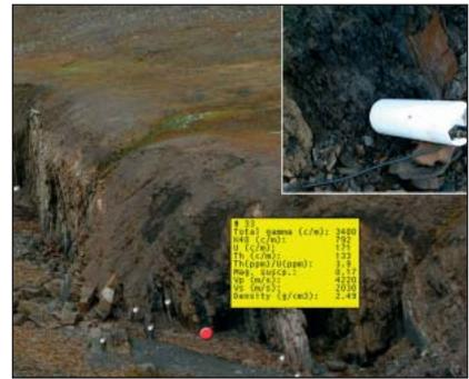
**Figure 6** At the Festningen, a 200 m section along the shore, a petrophysical log is measured and implemented in SVALSIM. In the image, white dots show where these data are sampled. When clicking on one of these dots with the left button, it turns red and shows the measurements in a yellow image (gamma measurements, magnetic susceptibility, velocities and density). Clicking on the right button shows a detailed image of the sampling spot.
