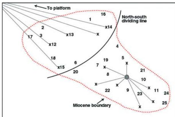
**Figure 3** Production (x) and injection (numbered) or planned injection (#/x). The numbering is arbitrary, as is the location in the bit-string.
