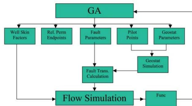
Figure 4 Schematic of the reservoir characterization process with ‘key variables’
