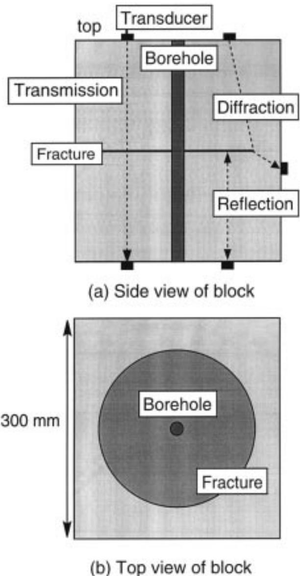
**Figure 3** Schematic experimental set-up for the acoustic measurements during hydraulic fracturing tests. A horizontal fracture grows perpendicular to a vertical wellbore. The dashed lines indicate the three types of records: transmission, diffraction and reflection.
