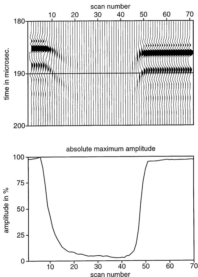
**Figure 13** S-wave transmission and its amplitude curve, measured 36 mm away from the borehole. In this case the fracture closes completely at the end of the experiment and the shear wave transmission is fully restored.
