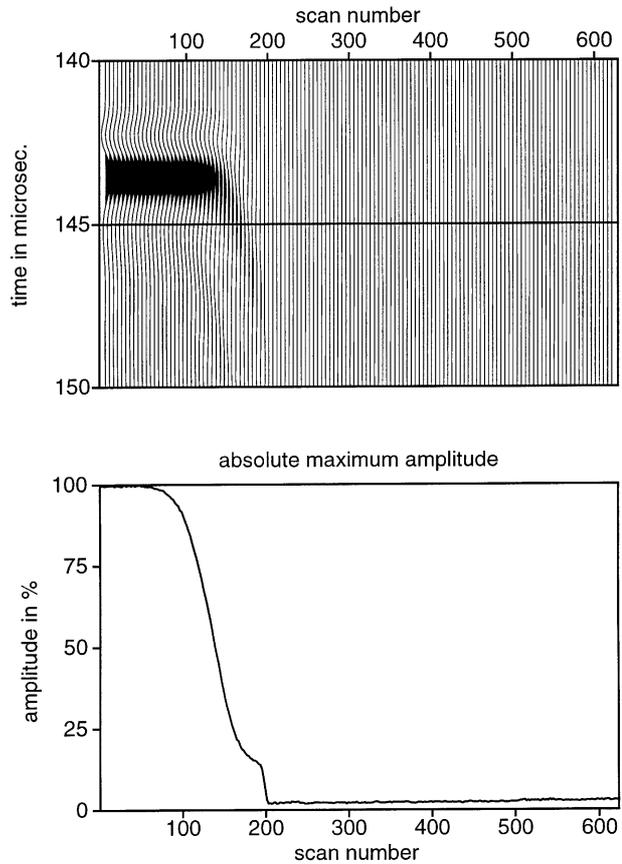
**Figure 12** S-wave transmission and its amplitude curve, measured 36 mm away from the borehole. Shear wave shadowing caused by the growing fracture is clearly visible.
