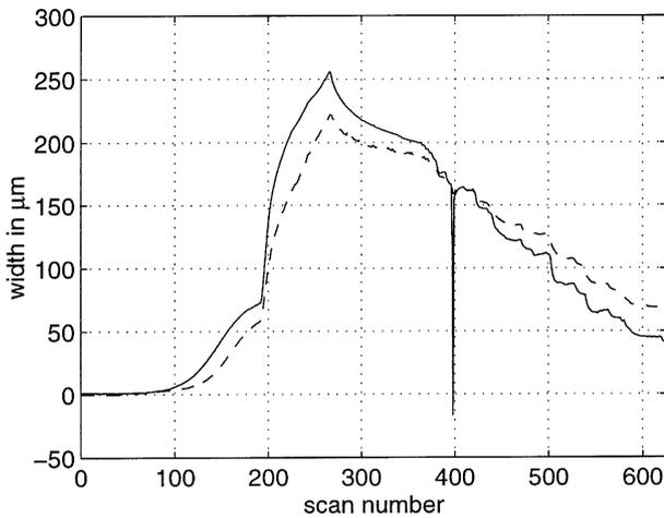
**Figure 11** Width profile across the fracture, measured inside the borehole with an LVDT. (solid line) The sudden drop in width around scan number 400 is a misreading by the LVDT caused by fluid flow inside the borehole. Estimated width calculated from transmission record of Fig. 10 at a position 36 mm radially away from the borehole (dashed line).
