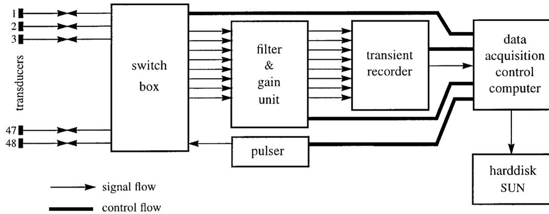
Figure 2 Schematic diagram of the acoustic data acquisition system.
