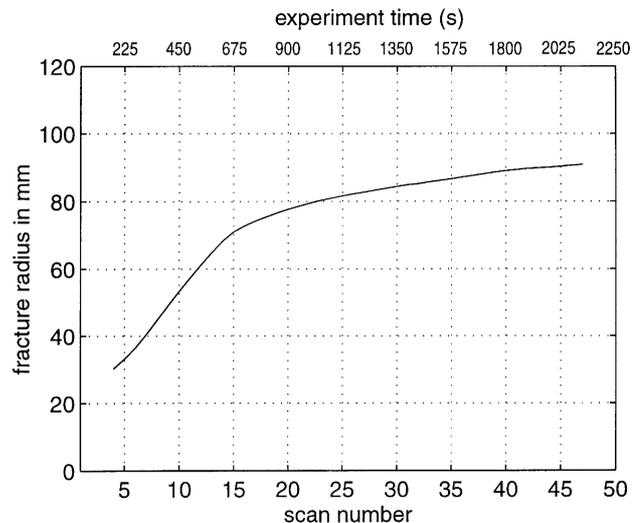
**Figure 5** Radius plot using the diffraction record of Fig. 4. The vertical axis denotes the fracture radius measured from the borehole, and the horizontal axis indicates increasing experiment time.
