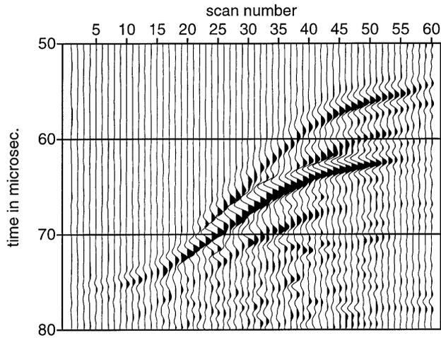
**Figure 6** Diffraction record made of a hydraulic fracture system consisting of multiple fracture wings, growing partly above each other.
