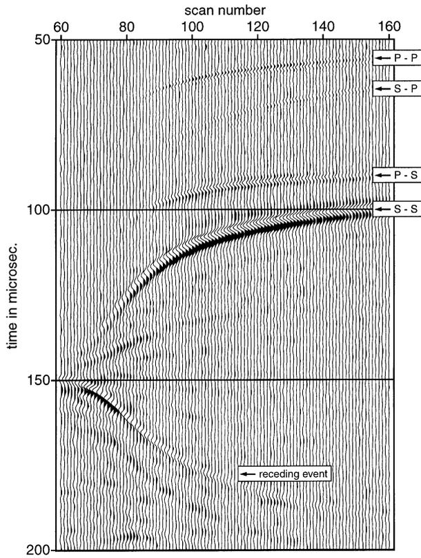
Figure 9 Diffraction record made with both sending and receiving S-wave transducers.
