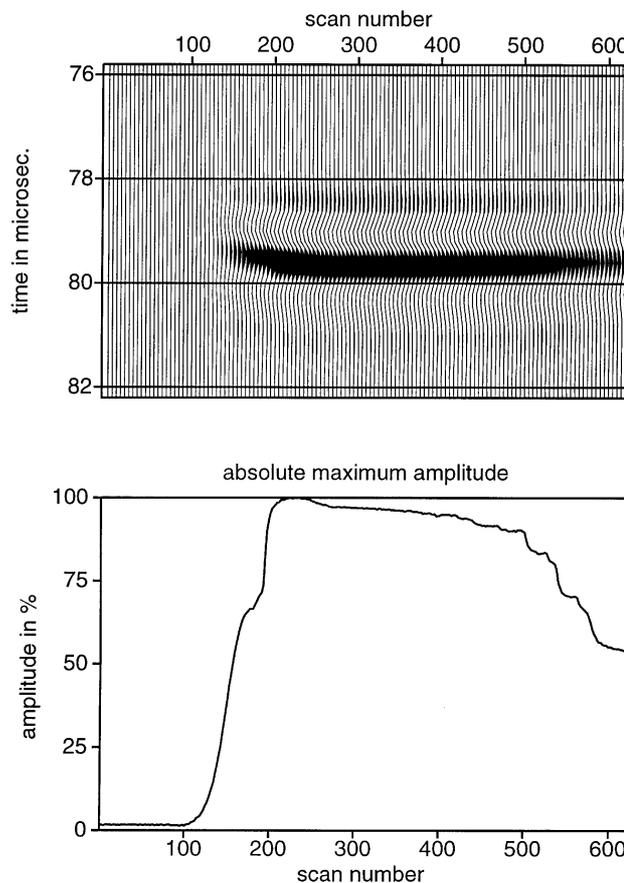
**Figure 14** P-wave reflection record and its amplitude curve, measured 36 mm away from the borehole. This record is from the same experiment as Figs 10–12. When the growing fracture intercepts the line of sight of the transducer, a reflection appears.
