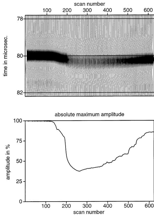
Figure 10 P-wave transmission and its amplitude curve, measured 36 mm away from the borehole. Dispersion effects caused by the growing fracture are clearly visible.
