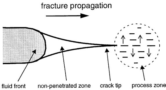
**Figure 7** Simplified and schematic overview of the fracture tip area.
