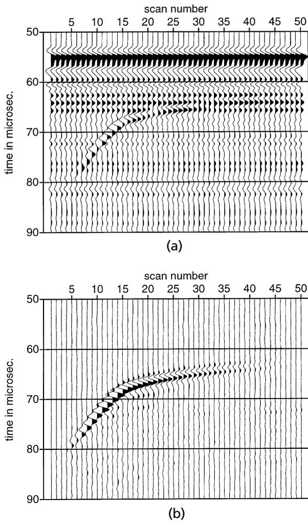
**Figure 4** (a) Original diffraction record for a fixed pair of transducers, with the vertical axis denoting travelttime and horizontal axis indicating increasing experiment time. (b) Same record after processing.
