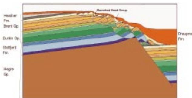
Figure 1 East-West cross-section through the Statfjord field.
