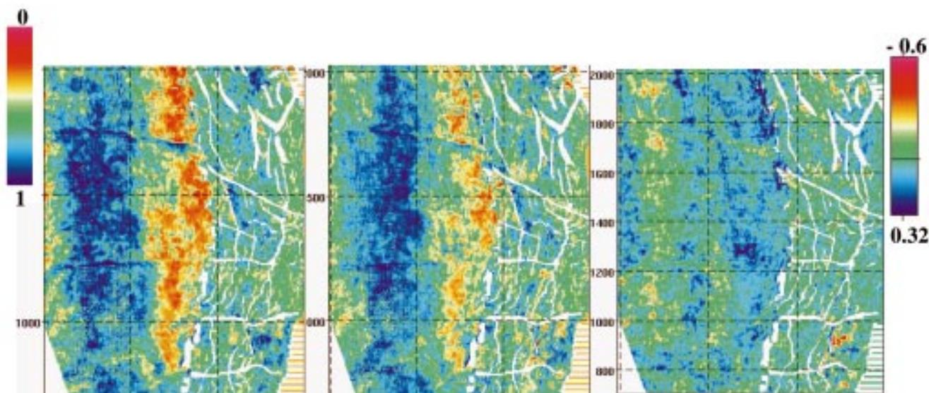
**Figure 5** Slices at 12 ms below top reservoir through 91 - and 97 saturation volumes (left and middle, respectively). At right the difference (97 minus 91) is shown. Blue indicates flooding with water.
