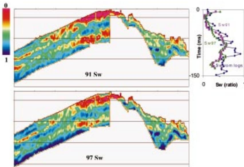
**Figure 4** East-West profiles through 91 - and 97 saturation volumes and a comparison between predicted and actual saturation at a blind test well drilled in 91. Red indicates oil, blue is water.
