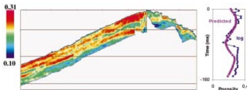
**Figure 3** East-West profile through the porosity volume and a comparison between predicted and actual porosity at a blind test location.
