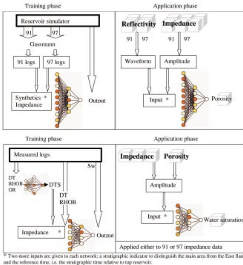
**Figure 2** Flow diagram porosity prediction (top) and water saturation prediction (bottom). Impedance means acoustic impedance, and mid and far angle elastic impedance.
