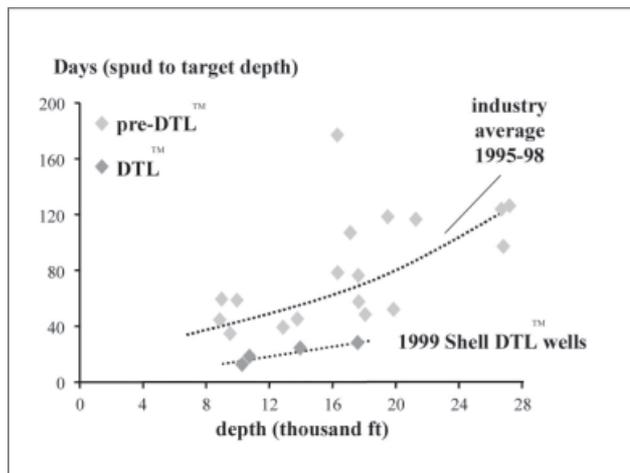
Figure 4 Drilling the Limit™—Shell Gulf of Mexico deep-water exploration drilling.
