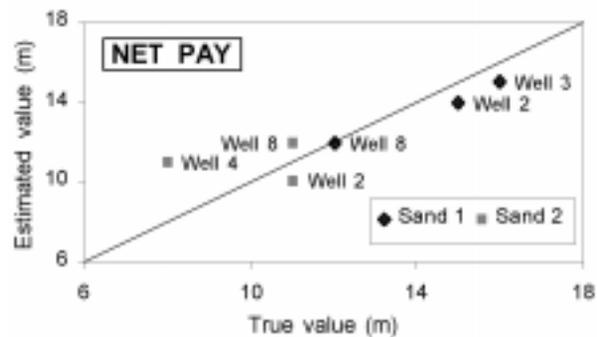
**Figure 11** Crossplot of estimated net pay from impedance vs. true (wireline measured) net pay for Sand 1 and Sand 2.
