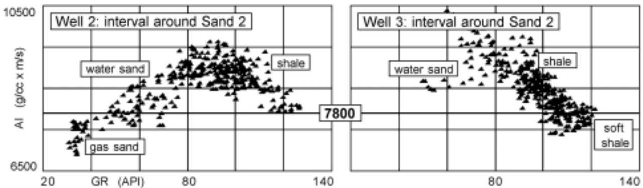
Figure 7 Sand 2: gamma ray vs. acoustic impedance crossplots from wells 2 and 3.
