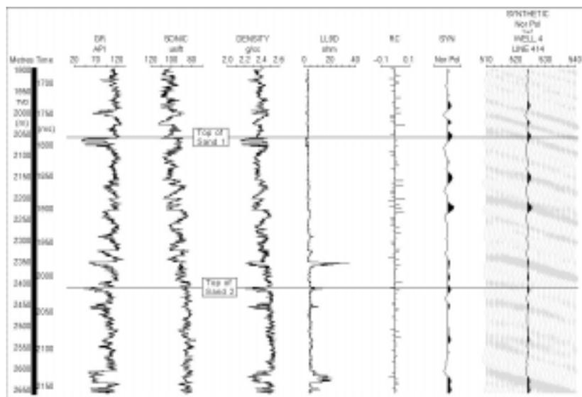
**Figure 4** Well 4: wireline logs, synthetic seismogram, and synthetic-seismic overlay.
