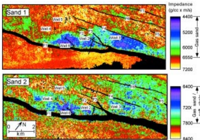
**Figure 9** Extracted impedance maps for Sand 1 and Sand 2. Symbols as in Fig. 1.
