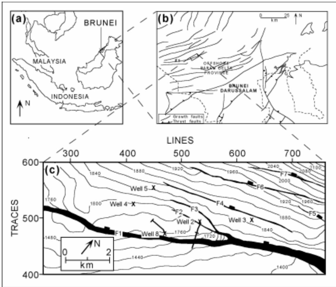
**Figure 1** Geological setting of the study area. (a) Regional location. (b) Structural trends of Brunei Darussalam (modified from James 1984). (c) Time structure map of the Sand 1 horizon. Contour intervals are 20 ms. F1 to F7 are faults. Well downhole positions marked by 'X'. Well trajectory indicated by line. Intersection location of well Sand 1 marker with interpreted time structure horizon indicated by tick along well trajectory.
