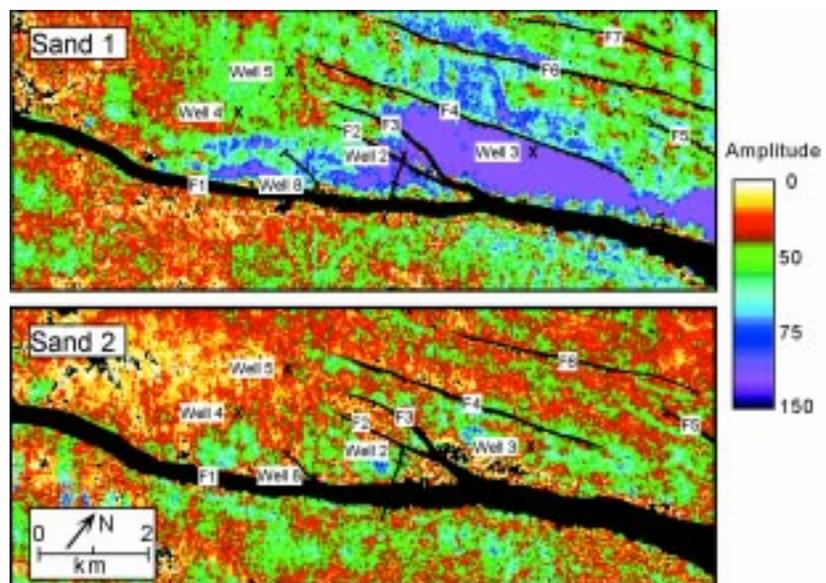
**Figure 12** Extracted maximum peak amplitude maps for Sand 1 and Sand 2. Symbols as in Fig. 1.
