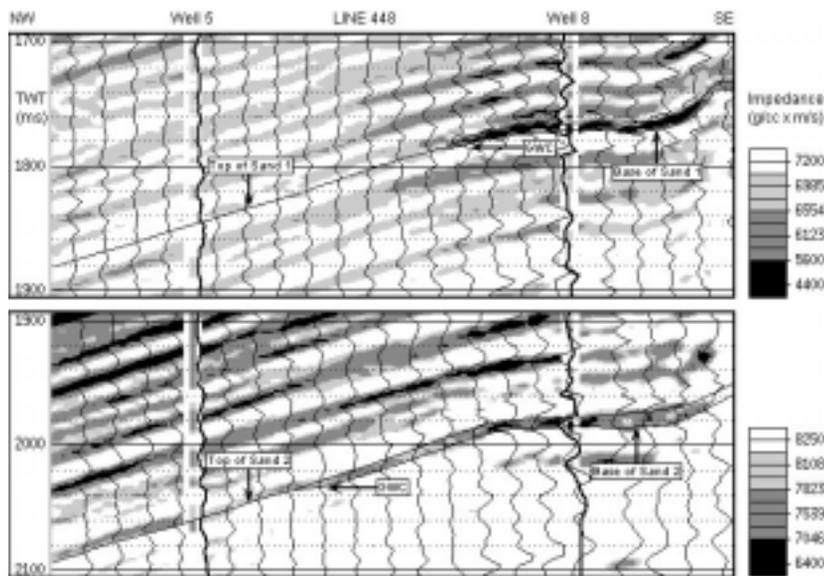
**Figure 8** Derived acoustic impedance sections interpreted separately for each sand. See Fig. 1 for line location.
