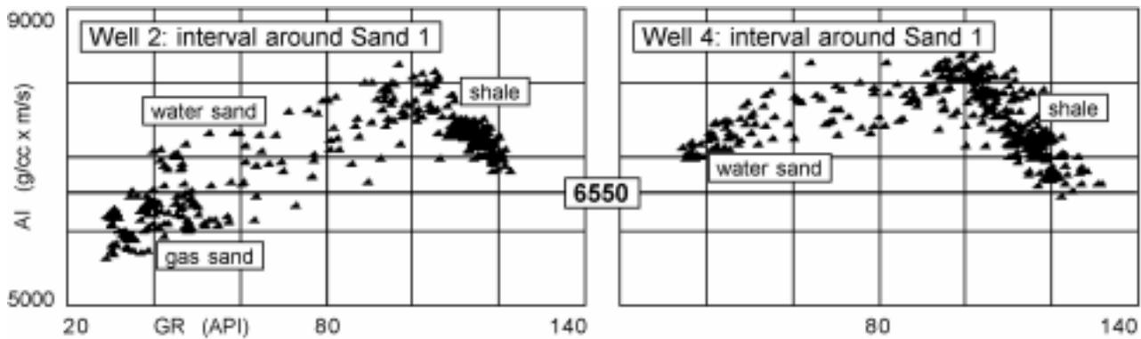
Figure 6 Sand 1: gamma ray vs. acoustic impedance crossplots from wells 2 and 4.
