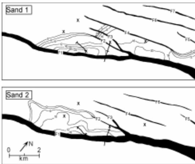
**Figure 10** Extracted net pay distribution maps for Sand 1 and Sand 2. Contour values in meters. Symbols as in Fig. 1.
