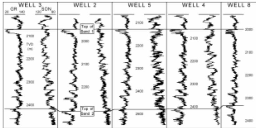
**Figure 2** Gamma ray and sonic log correlations for the two sands.
