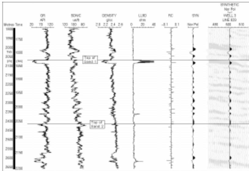
Figure 5 Well 3: wireline logs, synthetic seismogram, and synthetic-seismic overlay.
