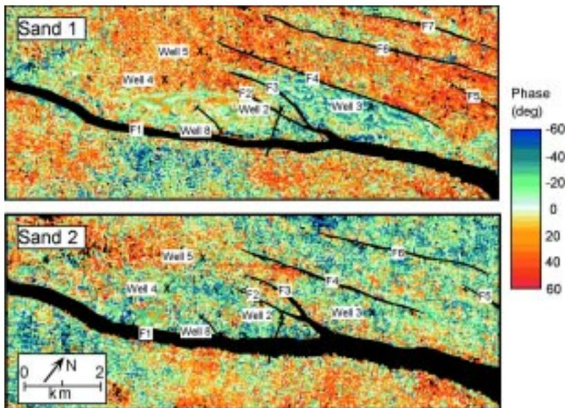
**Figure 13** Extracted average instantaneous phase maps for Sand 1 and Sand 2. Symbols as in Fig. 1.
