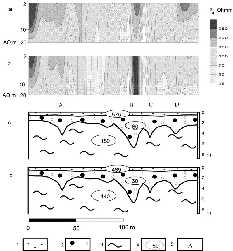
**Figure 3** Resistivity surveys data. a, b—pseudo-sections, obtained in April and May, respectively. c, d—results of data inversion, obtained in April and May, respectively; 1—non-saturated sand, 2—water saturated sand and gravel sand, 3—sandy clay, 4—resistivity values in Ohm-meters, 5—regions of high sand thickness.
