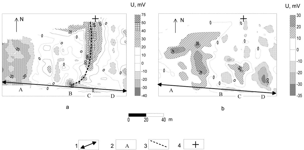
**Figure 4** SP maps of two surveys: a—obtained in April, b—obtained in May 1—sounding profile, 2—regions of high sand thickness, 3—anomaly due to filtration, 4—spring.
