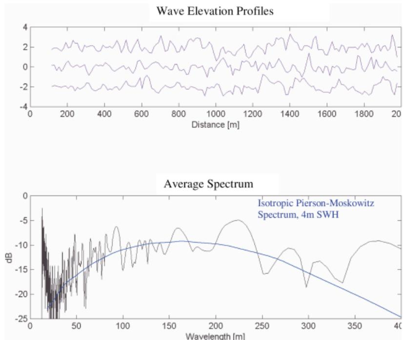
**Figure 4** Top: Wave elevation profiles from each streamer. They are vertically separated for visual clarity, and the vertical exaggeration is about 50 : 1. Bottom: Average wave number spectrum of the inverted sea surface profiles. The smooth blue line represents the isotropic Pierson–Moskowitz spectrum for a 4 m sea. There is reasonable agreement, and the dominant wave energy occurs around the same wavelength.
