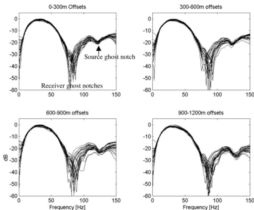
**Figure 2** Amplitude spectra of the isolated salinity reflection in Fig. 1. Each panels plots approximately 25 overlying spectra from increasing offsets. Top left: 0–300 m range, top right: 300–600 m range, bottom left 600–900 m range, bottom right: 900–1200 m range. The source ghost notch at around 125 Hz (6 m depth, and in this example heavily filled) is easily distinguishable from the receiver ghost notches (nominal depth 9 m), which show a spread of positions.
