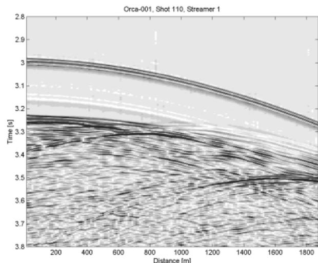
**Figure 1** Example shot record from streamer 1. The salinity interface reflection is the isolated event at 3.0 s TWT. Residual bubble energy from the airgun array is event at about 3.15 s TWT. The water bottom reflection is the event at about 3.25 s TWT.
