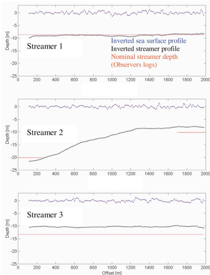
**Figure 5** Inverted streamer elevation profiles for the three streamers. The sea surface profiles (as shown in Fig. 4) are shown above each streamer on the same scale. The streamer profiles are smoothly varying compared to the sea surface profiles, and do not correlate with the sea surface shape. Note that there is no constraint in the inversion that forces this result. The nominal streamer depths as recorded on the observers' logs are shown in red.
