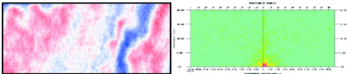
**Figure 9** The equivalent 3D time slice and Kx-Ky plot for one sweep/VP, 100 m Source line spacing. The acquisition footprint has been suppressed by the field geometry.
