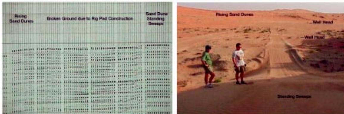
**Figure 2** Vibrator fleet traversing an area of ground previously subject to rig pad construction. There are apparent short period variations in the character of the first energy arrivals within individual VPs. The rightmost panel of 12 traces were recorded with no move-up between sweeps.
