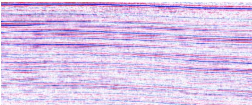
**Figure 5** Three sweeps/VP, 200 m source line spacing. Differential source elevation statics applied before sum of sweeps.
