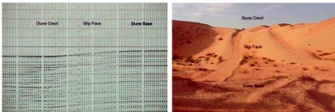
**Figure 1** Vibrator fleet traversing the slip face of a sand dune (left-to-right, dune crest-to-base). For scale, the object at the top of the left track is a Toyota Landcruiser. Note the approx. 60% decrease in amplitude of the traces from sweep positions as the vibrators move down the dune slip face. There is also 20 msec. differential arrival time across the twelve sweeps from a single surface VP.
