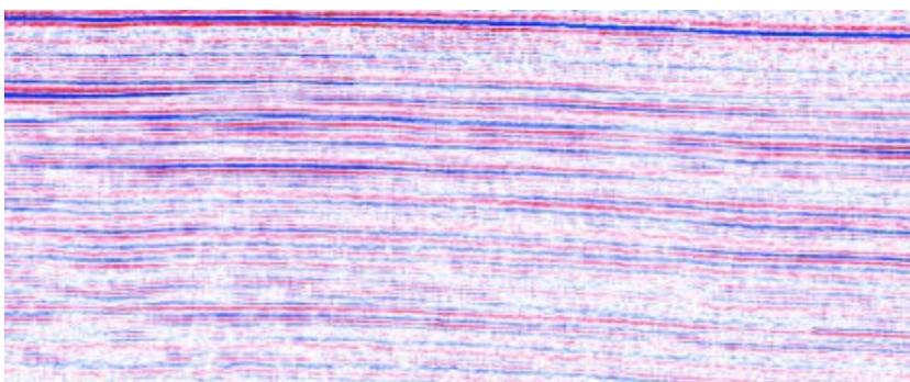
**Figure 4** Three sweep/VP, 200 m source line spacing. No differential source elevation statics applied before sum of sweeps.
