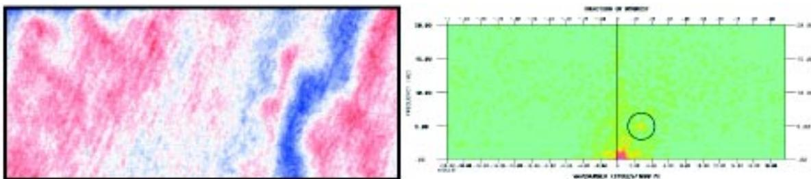
**Figure 8** A 3D time-slice and Kx-Ky plot from test volume of three sweeps/VP, 200 m Source line spacing. Differential Source elevation corrections were applied before summation. Some interference from an acquisition 'footprint' is evident. The circled area on the Kx-Ky plot indicates the corresponding energy concentration.
