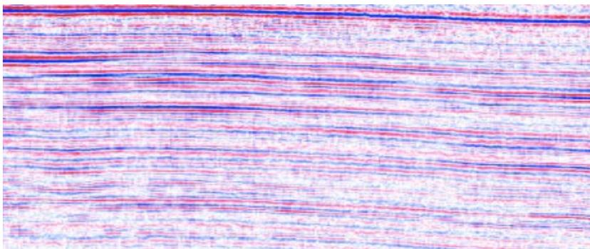
**Figure 3** Six sweeps/VP, 200 m source line spacing. No differential source elevation statics applied before sum of sweeps.
