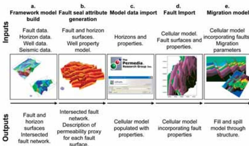
**Figure 5** Workflow to derive fault-controlled fill and spill through a field modelled using TrapTester and MPath. Fault attributes and the fault horizon framework and attributes exported from TrapTester form the basis of a realisation that incorporates the threshold pressure properties of the fault network within the percolation model.
