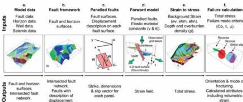
Figure 8 Prediction of small-scale fractures and faults is possible using geomechanically-based methods such as elastic dislocation modelling. Within TrapTester, elastic dislocation modelling is implemented in a straightforward workflow allowing prediction of fracture failure mode, orientation and density using the subsurface model data as input.
