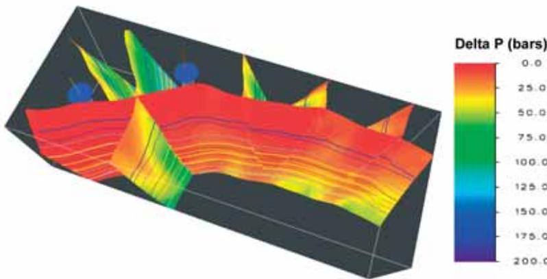
**Figure 4** The change in fluid pressure required to reactivate a fault can be mapped on the fault surface with a knowledge of the in situ stress system, pore pressure system and fault geometry. Faults with red colours require only a small pore pressure increase to reactivate and may be more transmissive to migrating, or leaking, hydrocarbons.
