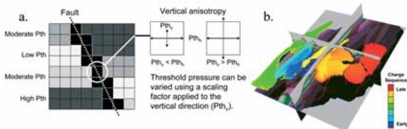
**Figure 6** a) The high-resolution MPath cellular model incorporates faults explicitly. Faults have lateral and vertical permeability and capillary properties. This allows description of the lateral and vertical flow within the fault zone. b) A realisation of fill and spill for one fill scenario in the Gullfaks field from the North Sea. Fill and spill are controlled by low capillary pressure windows on the fault plane.
