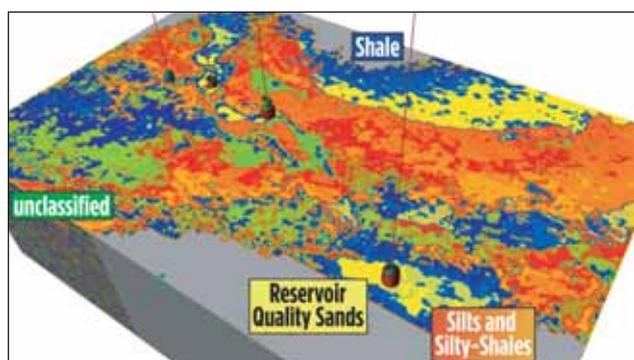
*Seismic volume - calibrated to geologic properties*
