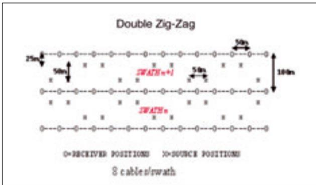
Figure 7 Double Zig-Zag field configuration (x=shot, o=receiver).
