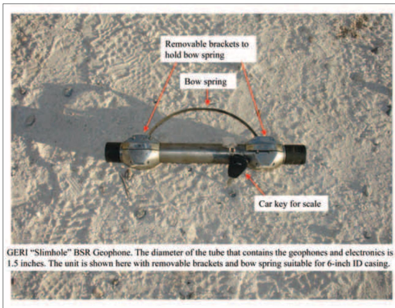
**Figure 2** Slimhole borehole sonde. The three-component geophone sonde is shown with a clamping device attached. The weight of the device shown is about 2 Kg and as many as 480 of these sondes can be deployed on a fibre augmented wireline. There is effectively no time delay between the geophones and the recording system with the maximum number of sondes on the wireline.
