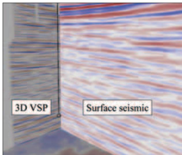
**Figure 1** Comparison of 3D VSP and surface seismic images. Two abutting slices from a 3D VSP image (left) and a 3D surface seismic survey (right) are shown. Discontinuous sands and shales are imaged by both datasets but the 3D VSP has twice the frequency content of the surface seismic data, thus small faults and stratigraphic changes that control production are more easily identified in the 3D VSP image.
