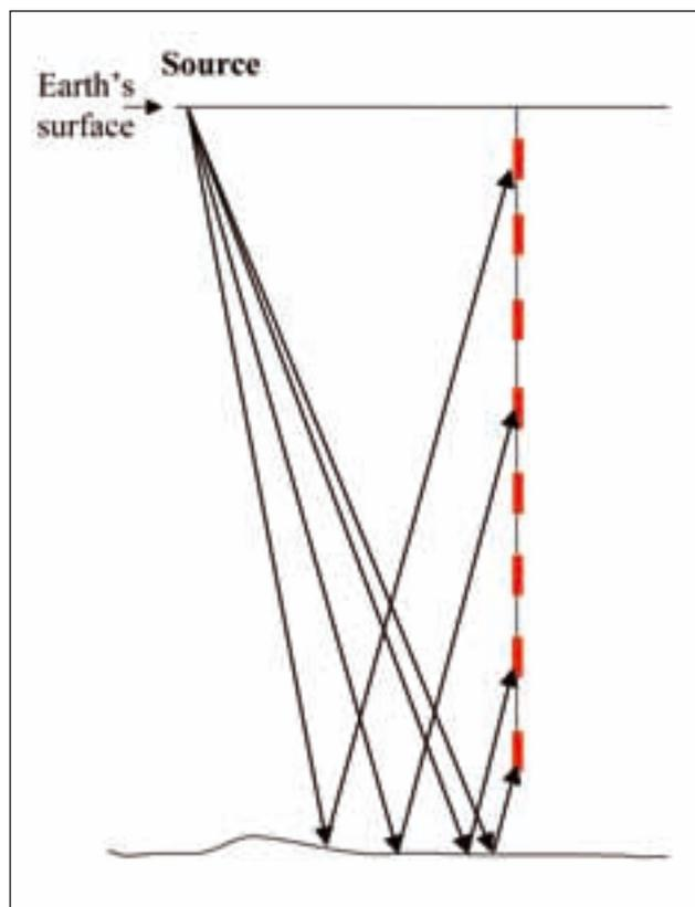
**Figure 3** Offset VSP geometry. The asymmetric downgoing and upgoing ray paths of VSP geometry result in the reflection points being a function of the source and receiver positions and the velocity field rather than the common mid-point assumption of surface seismic data. The asymmetry imposes greater complexity in reflection velocity analysis than is encountered in surface seismic data processing. The higher frequency of VSP data imposes an additional requirement on velocity field accuracy.
