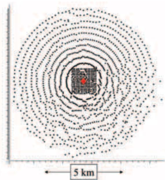
**Figure 6** 3D VSP source point map. A source point map for a recent 3D VSP shows dense source spacing near the receiver well at the centre of the survey. The roughly circular source pattern at larger offsets provides uniform reflection coverage. The target depth range for this survey was as much as 5000 m.
