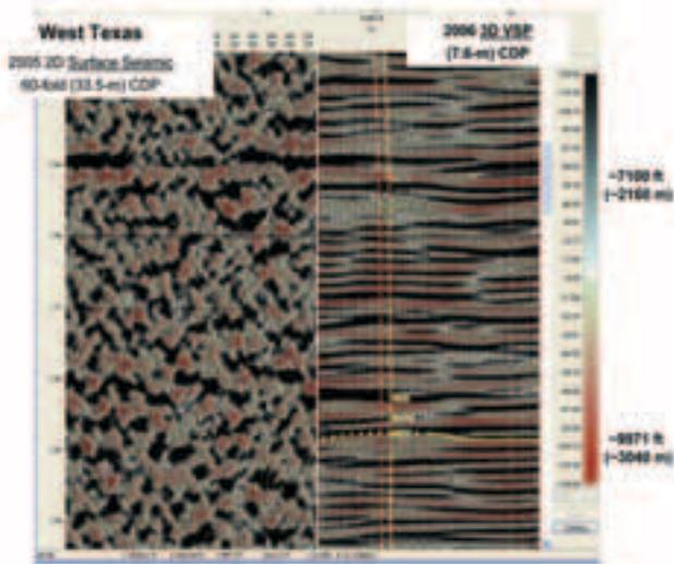
**Figure 5** Surface seismic and 3D VSP comparison. A recently-recorded 2D seismic image (left) near the 3D VSP well is shown for comparison of data quality with the 3D VSP data (right). This area in West Texas is a difficult data area for surface seismic data but apparently much less so for the 3D VSP technique.
