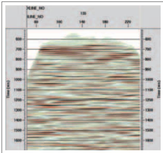
**Figure 4** West Texas 3D VSP image. This image is from a 3D VSP in West Texas. The dataset was recorded in January 2006 and is being used to pick step out drill locations from the 3D VSP well.
