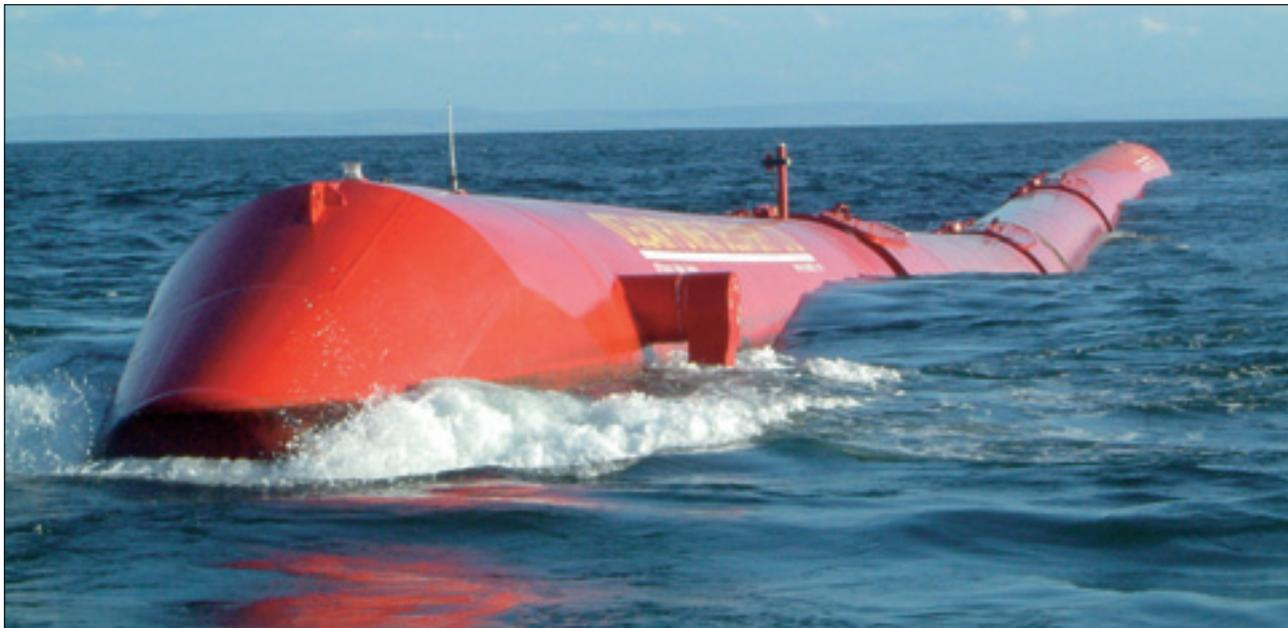
**Figure 3** Ocean Power Delivery's Pelamis wave power device undergoing sea trials. Pelamis is supported by Norsk Hydro. (Photo reproduced by permission of Ocean Power Delivery Ltd.).
