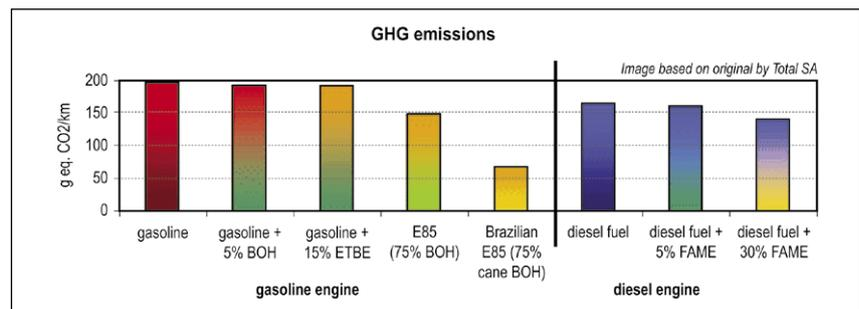
Figure 1 Emissions reduction using biodiesel (from Total, 2007) (ETBE - ethyl-tertiary-butyl-ether; FAME - fatty acid methyl ester).
