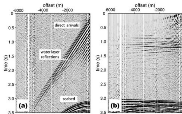
**Figure 3** Shot records to illustrate signal/noise characteristics and effect of processing. (a) Shot record of raw data (b) Same record after noise removal and NMO correction using constant velocity. Data may require further noise suppression before detailed analysis.
