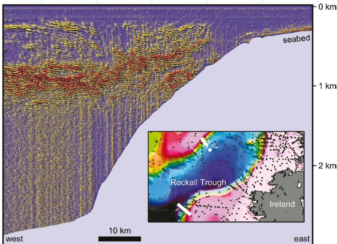
**Figure 1** Depth-converted seismic reflections from the water column within Rockall Trough, west of Ireland. A variable-area display to show the reflections (grey-scale) is superimposed on an amplitude envelope indicating reflection strength (red colour = high amplitude). Inset shows line location on SE Rockall margin with seafloor topography, and also the locations of oceanographic CTD (conductivity-temperature-depth) measurements (circles).
