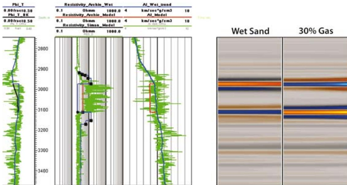
Figure 8 Synthetic seismic gathers show strong amplitude difference between wet case (left) and the non-commercial 30% gas case (right).
