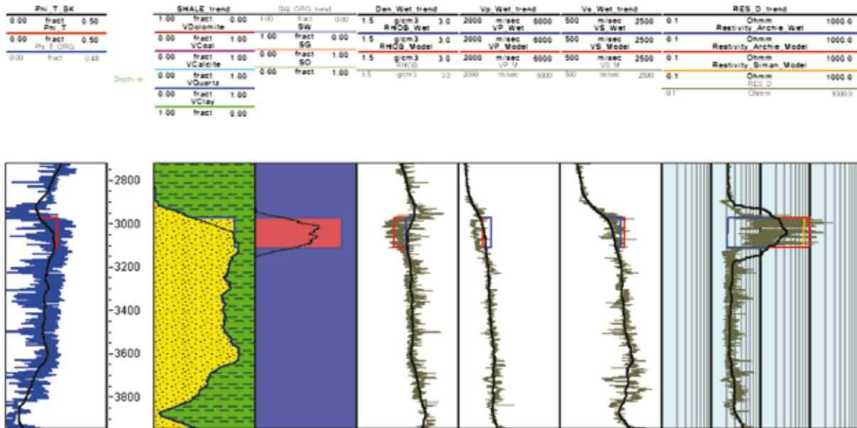
Figure 5 Fine scale (grey) and smoothed (black) well log curves (6707-10-1 well) and modelled gas sand at about 3000 m depth.
