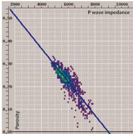
**Figure 11** Crossplot of porosity versus P wave impedance for the reservoir interval. There is a well-defined linear relationship in the reservoir unit.
