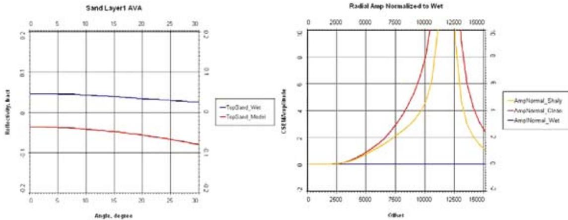
Figure 7 (left) Reflectivity versus angle of incidence for wet (blue line) and 85% gas case (red line); (right) Normalized radial CSEM amplitude versus source-receiver distance for wet (base case) and 85% gas case. Note that the difference between the wet and gas case CSEM amplitude ranges from a factor of five for shaly sand (orange line) to a factor of eight for clean sand (red line) at the maximum spacing of 10,000 m.
