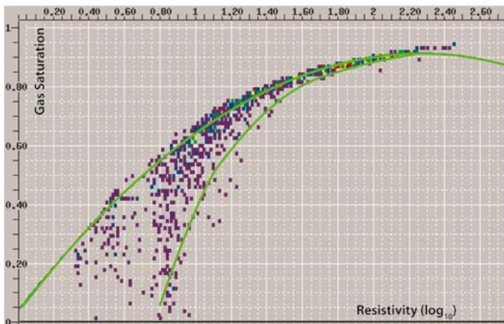
**Figure 12** Gas saturation versus  $\log_{10}(\text{resistivity})$ . The green line represents an upper bound on the gas saturation, and equally well a lower bound can be obtained from the lower limit of the point cloud. The scatter between them is partly due to the varying clay content within the reservoir sands. At high saturations the uncertainty in the saturation estimate is low, whereas at lower saturations it becomes greater.
