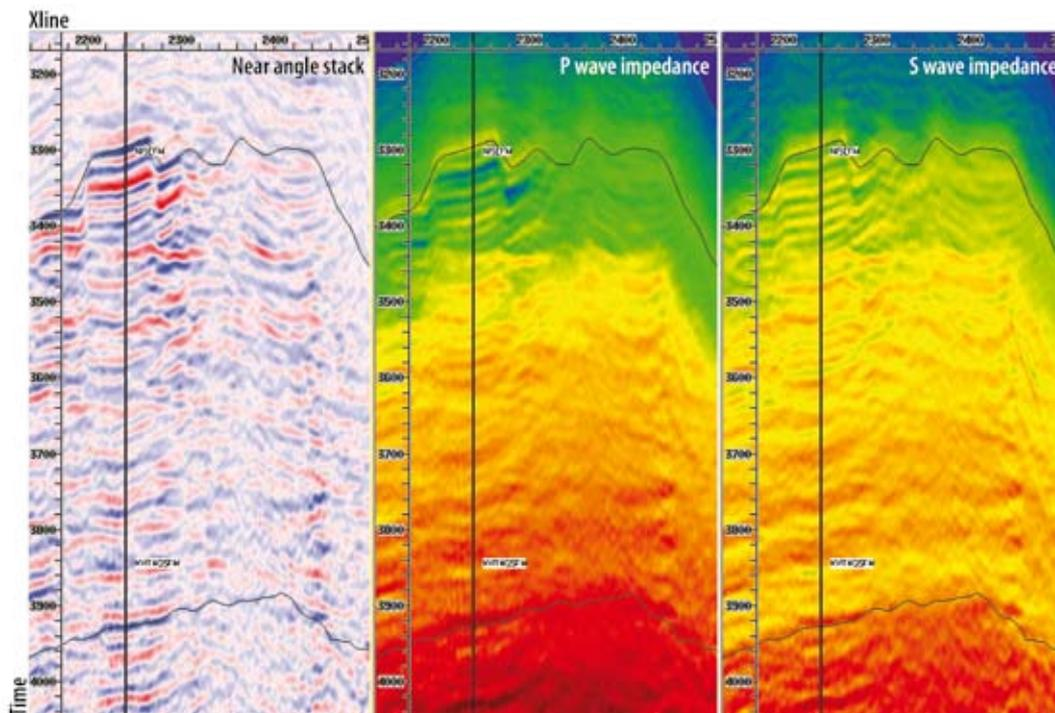
Figure 10 from left to right: Near angle stack, P wave impedance, S wave impedance. The top reservoir pick and the well location are also shown. The gas-water contact is evident in the seismic data and is brought out clearly as the green-yellow transition in the P wave impedance.
