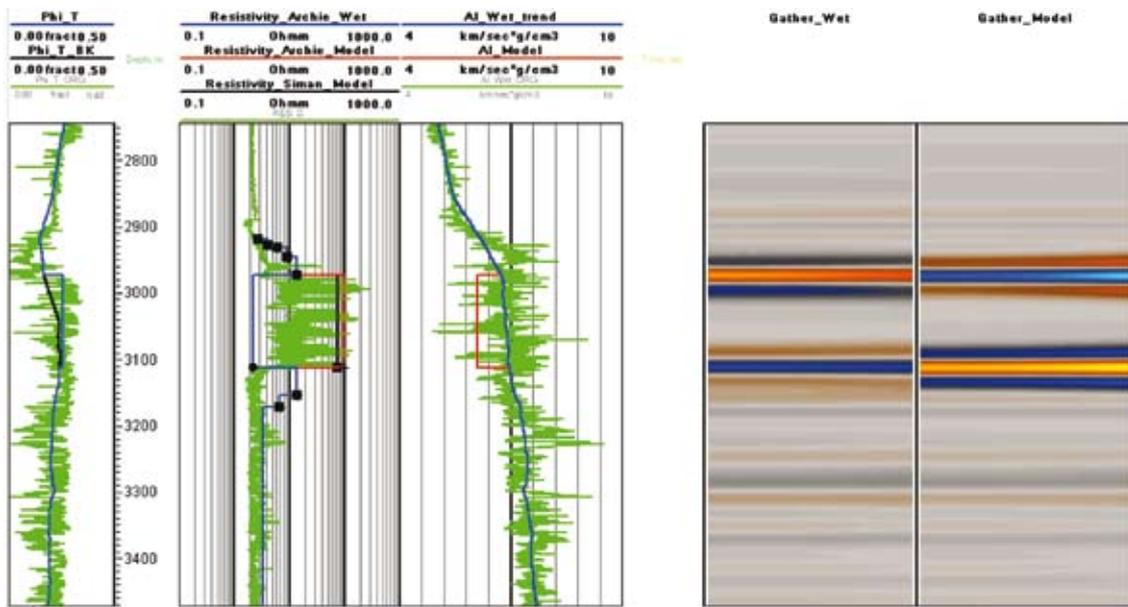
Figure 6 Synthetic seismic gathers show strong amplitude difference between wet case (left) and 85% gas case (right). Orange colours in the gather indicate positive amplitude (low AI over high AI), blue colour indicates negative amplitude (high AI over low AI).
