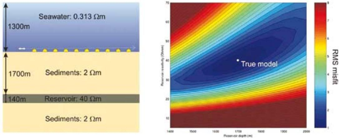
Figure 2 Left panel: simplified 1D resistivity model based on the structure of the Luva gas reservoir. CSEM responses at 0.25 Hz, 0.75 Hz, and 1.25 Hz were contaminated with 5% noise to produce a synthetic dataset. Right panel: Misfit of the model response to the synthetic data as a function of target layer resistivity and depth. There is a clear trade off in these parameters.
