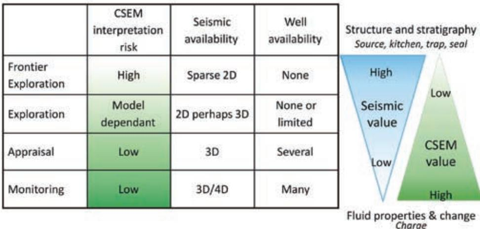
Figure 2 Schematic illustrating the applicability of CSEM and seismic methods across the oil field life cycle.
