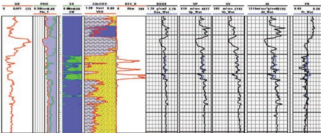
Figure 1 Well log suite illustrating that the hydrocarbon saturated zone is clearly delineated as a region of high resistivity (red curve in the fifth track). In contrast the acoustic and elastic curves (right four tracks) show only a small difference between the water saturated (blue) and hydrocarbon saturated (black) cases.
