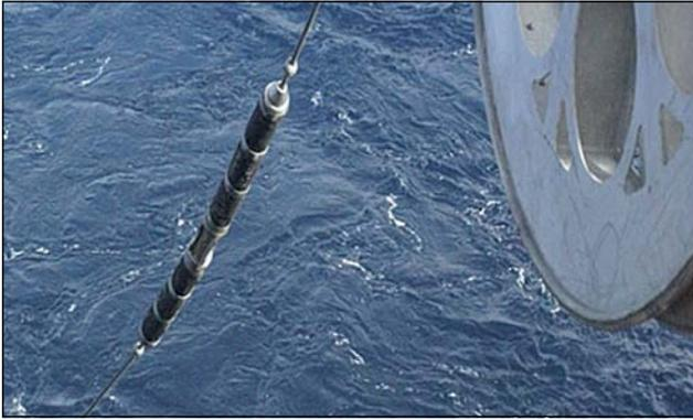
Figure 3 Cable for the OBC system being deployed.
