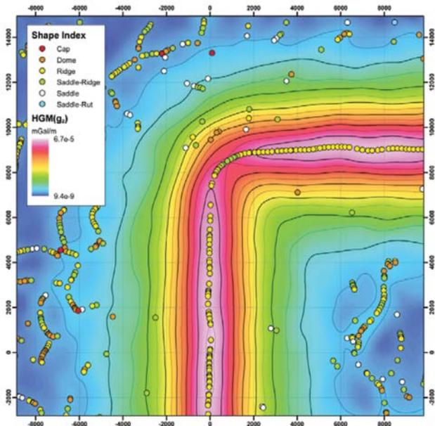
**Figure 5** Depth estimates for a semi-infinite slab of finite width (18 km in the  $y$  direction) and thickness 100 m lying flat at a depth of 1 km below the observation points. The excess density is  $+100 \text{ kg/m}^3$ . The contours of the HGM of  $g_x$  with noise added and upward continued by 1 km are shown for the northwest corner of the sheet only. Depth estimates are plotted as coloured dots depending on their associated Shape Index.
