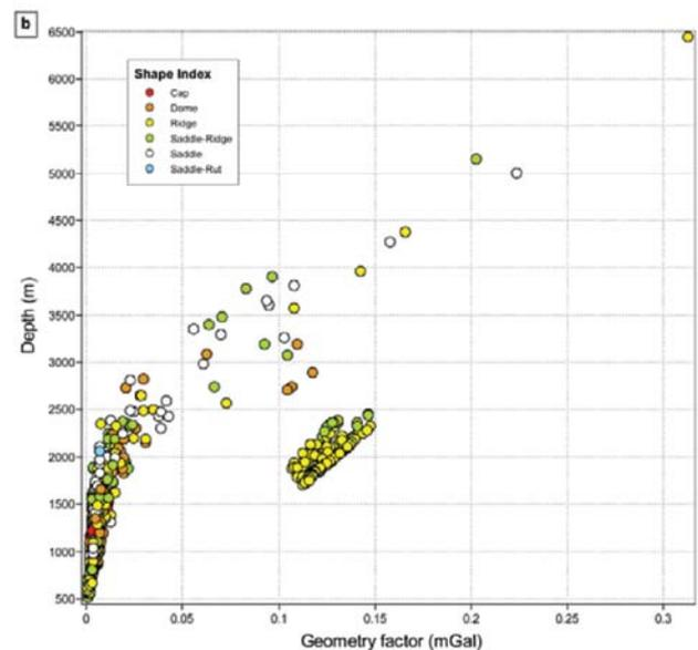
**Figure 6** Discrimination of depth estimates using the Shape Index and the geometry factor in the case of the thin sheet described in Figure 5. (a) Depth as a function of SI. The colours are the same as in Figure 5. (b) Depth as a function of the geometry factor. The source has a theoretical  $\alpha$  value of 0.13 mGal. The correct depth is 2 km.
