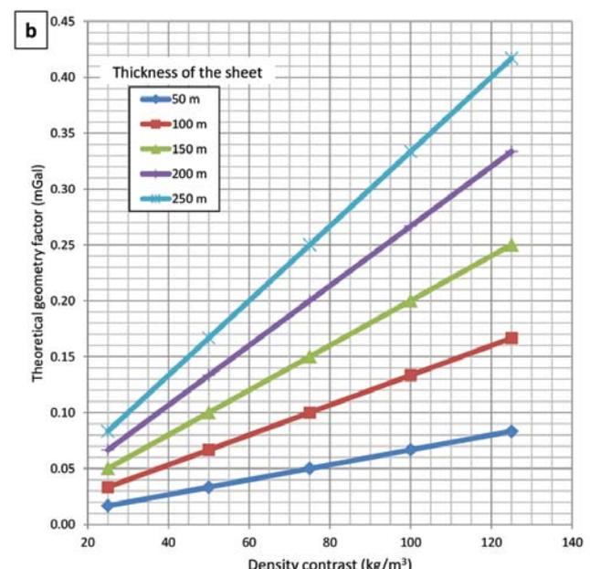
Figure 2 Theoretical geometry factor as a function of density contrast. (a) horizontal cylinder; (b) thin sheet.
