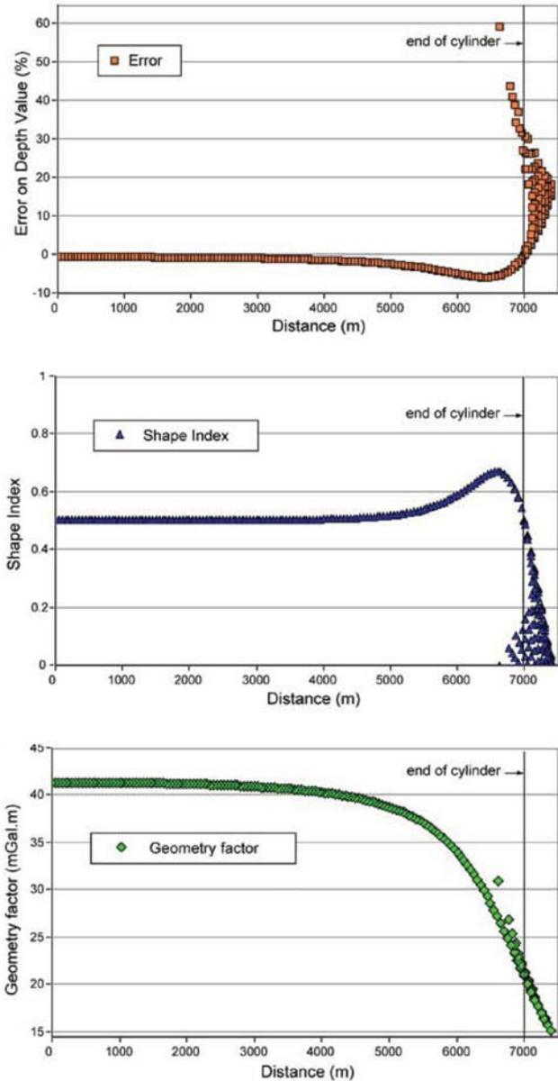
**Figure 4** Depth estimates for a horizontal cylinder as defined in Figure 3. The error on the calculated depth, the Shape Index and the calculated geometry factor are plotted against the distance along the y axis. The northern end of the cylinder is at  $y = 7$  km.
