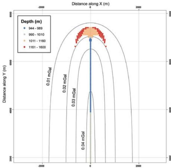
**Figure 3** Depth estimates for a horizontal cylinder of finite length (14 km) and radius 100 m buried at a depth of 1 km below the observation points. The excess density is +100 kg/m<sup>3</sup>. The plot only shows the northern half of the gravity anomaly. Depth estimates are plotted with points coloured as a function of depth.
