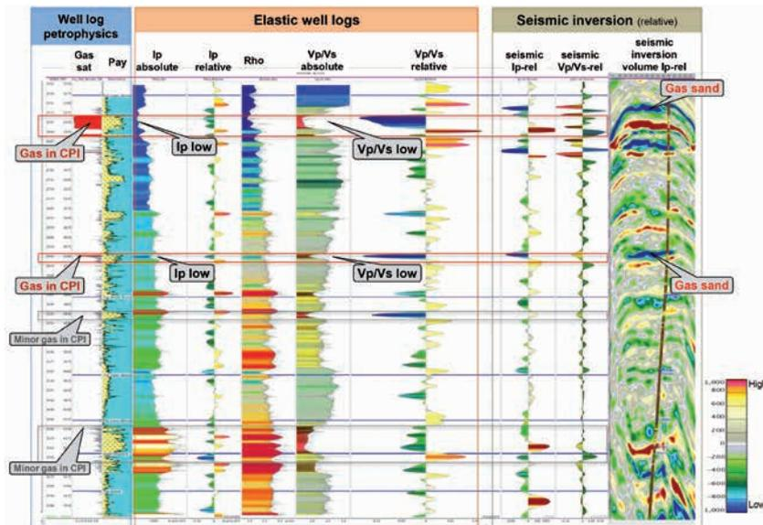
Figure 5 An example of a well log elastic attribute to seismic inversion volume comparison display showing the correlation between the presence of hydrocarbons and the seismic inversion volume responses.
