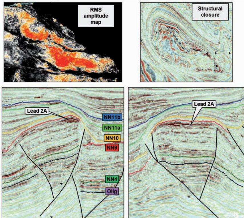
**Figure 7** An example of a lead identified using the sequence stratigraphic interpretation of the full stack seismic data. In this example, the bright amplitudes immediately below the NN9 sequence boundary are likely to be lowermost shoreface sandstones of the highstand systems tract while the sealing sediments above are likely to be deeper water transgressive mudstones.
