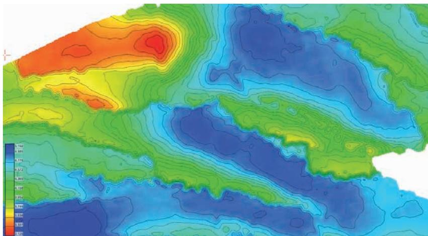
**Figure 4** An example of a two-way time horizon surface indicating the fault orientations and structures of the toe-thrust and diapiric shale zones. It is these structures that provide the migration pathways and trapping mechanisms for the encountered hydrocarbons.
