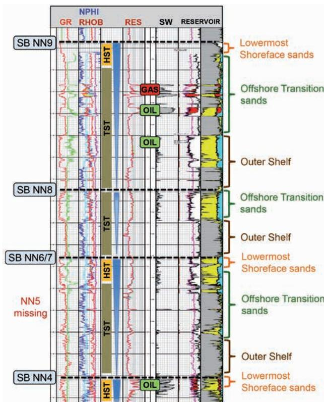
Figure 2 An example of a processed, workstation-ready well log from the study showing the sequence stratigraphic and depositional environment interpretation together with encountered hydrocarbons.
