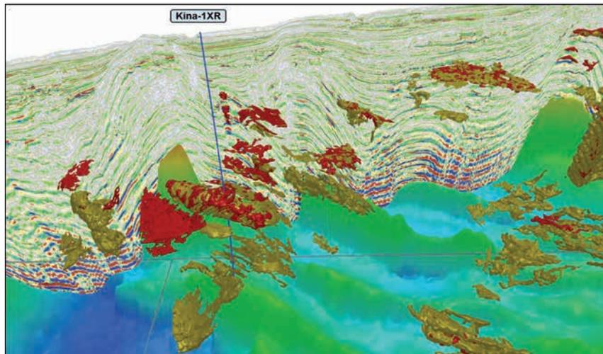
**Figure 8** An image showing the reservoir geobodies extracted from the seismic inversion volume together with the location of the Kina-1XR wellbore. A number of stacked, undrilled targets can be seen.
