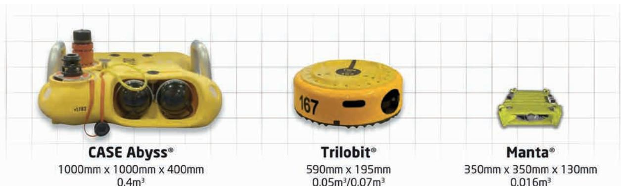
Figure 3 The evolution of deep water nodes. Three deep water ocean bottom nodes displayed to scale which have decreased in size over time, directly impacting ROV deployment efficiency.
