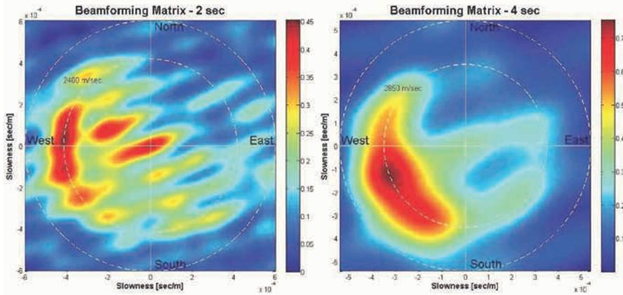
**Figure 2** Results of the beamforming analysis for 2 s (a) and 4 s (b) periods. The phase velocities of the maximum amplitude signals are displayed with white dashed circles.
