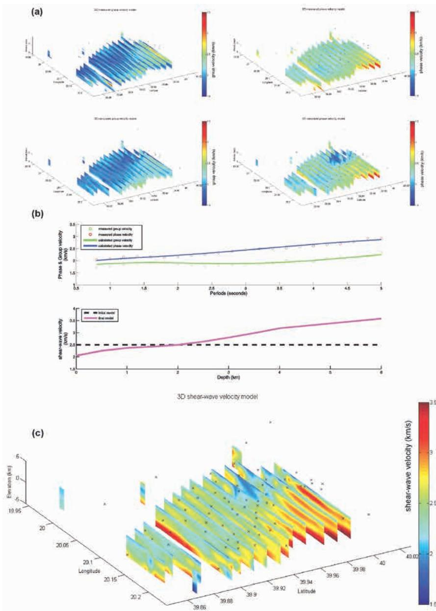
**Figure 6** a) 3D measured phase and group velocity models in comparison to the calculated ones, derived by the joint inversion. b) Example of jointly inverted local dispersion curves and the corresponding 1D shear wave velocity model. c) 3D shear wave velocity model of the study area.
