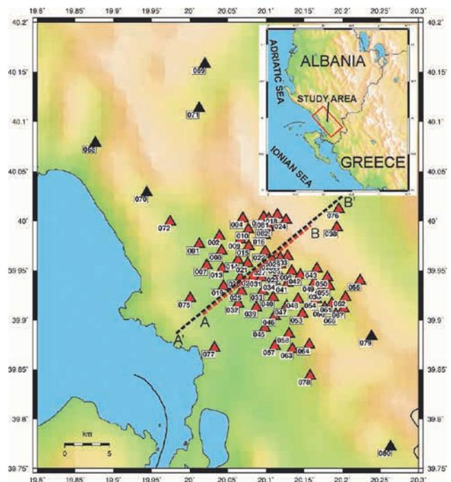
**Figure 1** Map of the study area and seismic stations (triangles) deployed during the second phase of a Passive Seismic Tomography survey performed in the area by Seismotech during 2011-2012. The stations used for the present study are displayed with red triangles. The dashed black and red lines denote the location of the geological cross-section and the extracted shear-wave velocity cross-section, respectively, shown in Figure 7.
