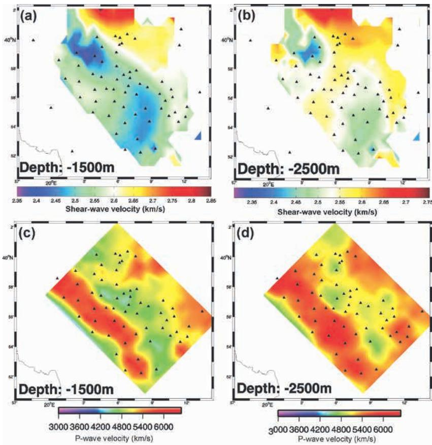
**Figure 8** Horizontal cross-sections through the 3D shear-wave velocity model at (a) 1500 m, (b) 2500 m and tomographic models of P-wave velocities around the Delvina area derived by a previous Passive Seismic Tomography survey. P-wave velocity models correspond to the same depths (c) 1500 m and (d) 2500 m.
