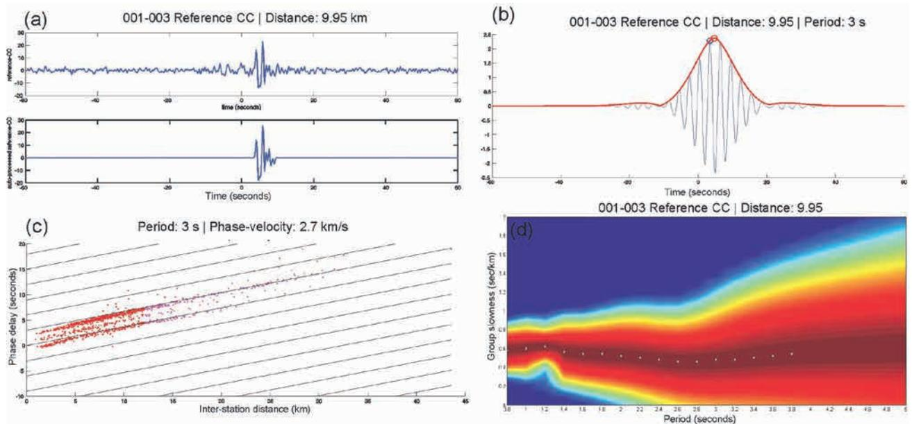
**Figure 4** Examples of a) signal's isolation from the reference CC function, b) initial estimation of group and phase delay on a filtered signal at 3 s period, c) diagram of the measured phase delays versus source-receivers inter-station distances (red and magenta dots correspond to inter-station distances less and greater than 1.5 wavelength, respectively) and d) Frequency - Time diagram. White crosses represent the maxima picked by the above mentioned automatic technique.
