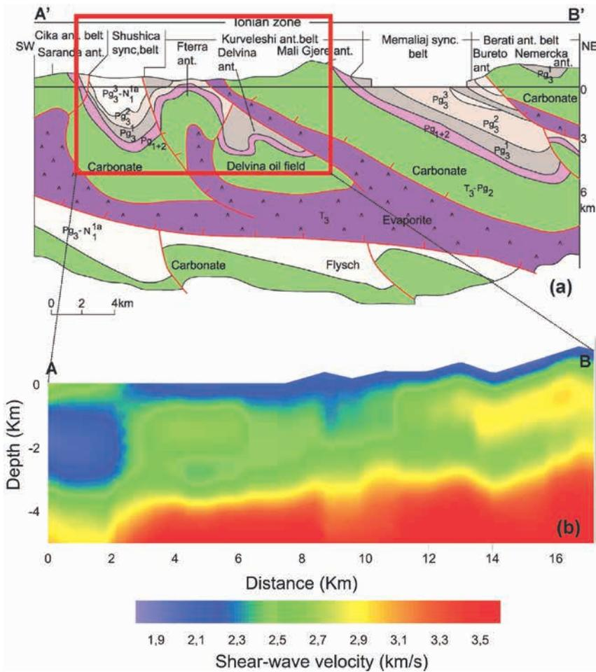
**Figure 7** (a) Schematic geological cross-section through the Delvina area (A'B'). (b) Vertical cross-section through the shear-wave velocity model derived from the depth inversion (AB). The spatial correspondence between the shear-wave velocity cross-section and the geological cross-section is depicted by the red rectangle (7a). The geological cross-section is from Velaj (2015). See Figure 1 for the cross-sections' location.
