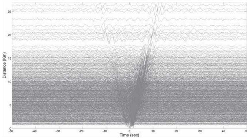
**Figure 3** Cross-correlation functions filtered between 0.16 and 1.2 Hz sorted by increasing inter-station distance.
