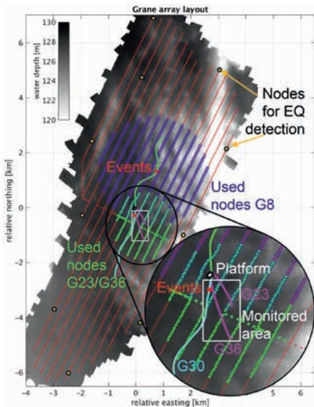
**Figure 1** Grane PRM field layout (red lines) showing the used nodes (green) for microseismic real-time surveillance of the injector wells G23 and G30 (magenta lines). The well path of G30 is also indicated (cyan line). Blue nodes indicate nodes used for the study of events from the G8 well (green line). Yellow stars indicate stations currently used for EQ detection. Bathymetry map in the background. Red dots indicate the location of events discussed in this paper.
