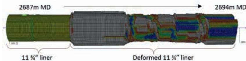
**Figure 3** Multi-finger caliper of deformed 11 3/4-inch liner in well G8.
