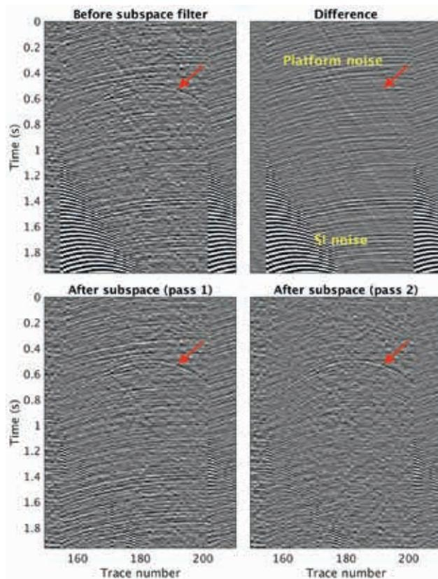
**Figure 2** Subspace filter application to raw data (top left), contaminated with SI (suppressed by first pass (bottom left)) and platform noise (suppressed by second pass (bottom right)). The difference image (top right) shows that the microseismic event (red arrow) is not touched by the filter. A 2-45 Hz bandpass and FX median filter have been applied to the raw data.
