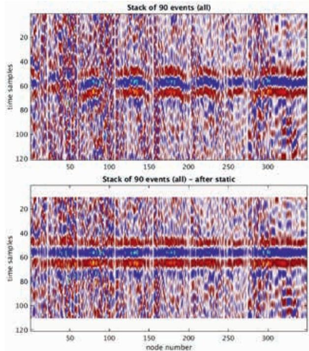
**Figure 9** Stack of 90 events, which origin from the same voxel, prior (top) and post (bottom) static correction.
