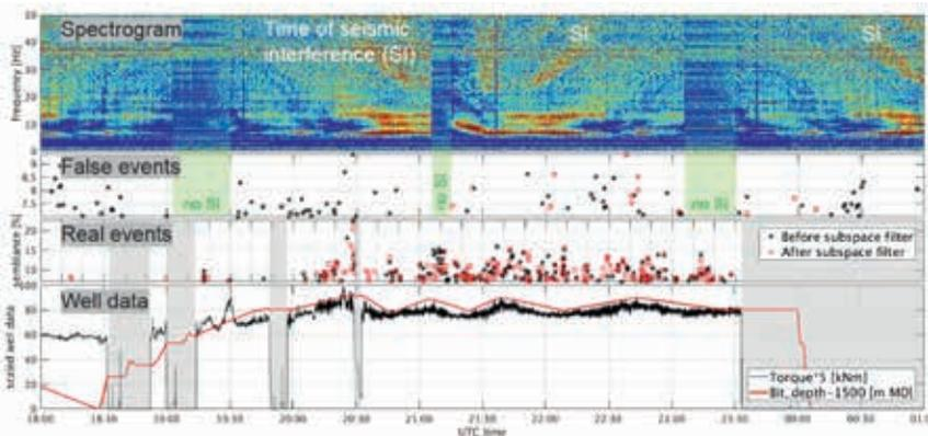
**Figure 8** Microseismic events detected during the P&A operation in G30. The spectrogram (top) shows the ambient noise with periods of seismic interference (SI). False and real microseismic events are shown with and without application of the subspace filter (middle panels) and well operation data (bottom).
